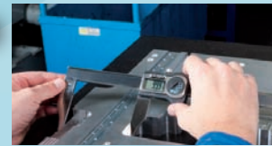
Center to center measurement using a caliper with external jaws
