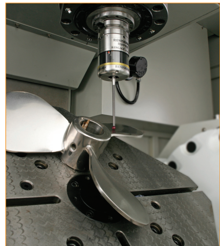
RMP600 probe inspecting a component, with RMI receiver / interface in the background
