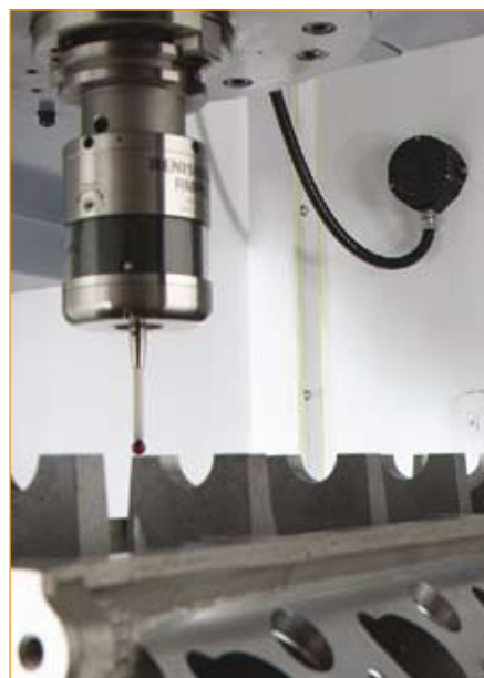
RMP60 probe inspecting a component, with RMI receiver / interface in the background
